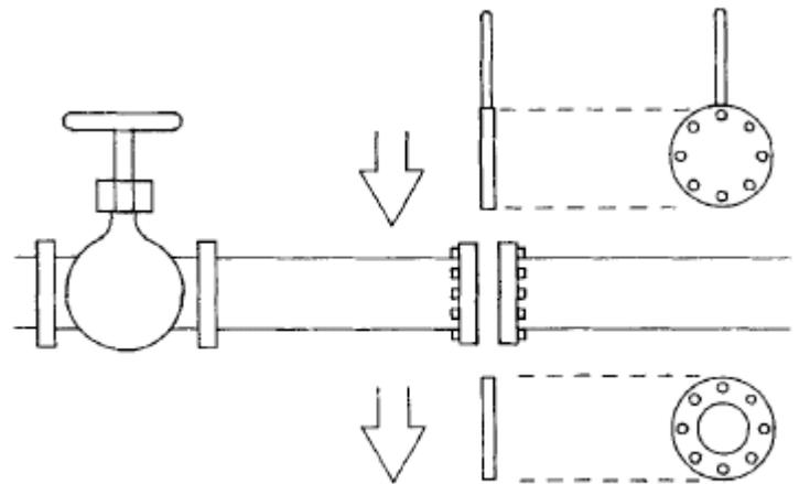
**Method of Blanking Hydraulic/Pneumatic Lines**
