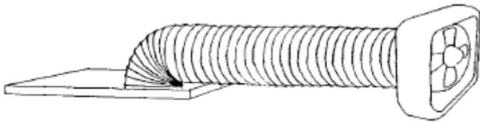
**Ventilating with Fan and Trunk Hose**
